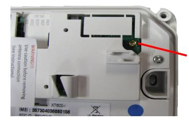
19" Pigtail Right-angle MMCX plugs in the 'RADIO' location on the XT Control Panel. This plug must not get loose or you will lose reception.
